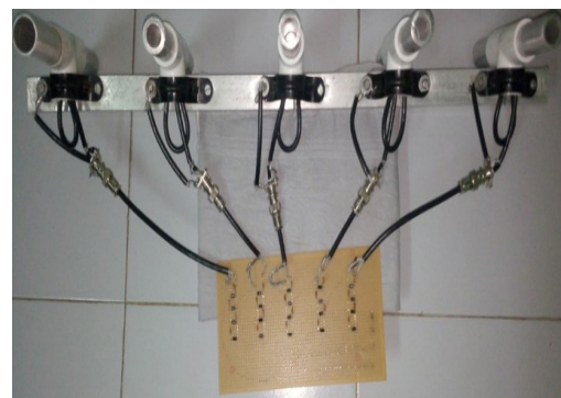
Fig 9. Hardware of the RF-DC Conversion circuit with Array
