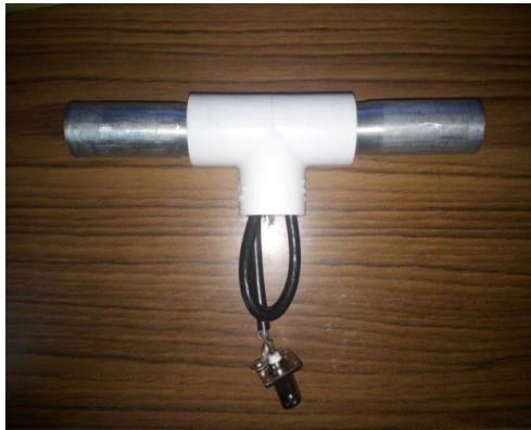
Fig 3. Single fabricated dipole antenna 13.8cm
